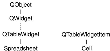
**Figure 4.1.** Inheritance trees for `Spreadsheet` and `Cell`
