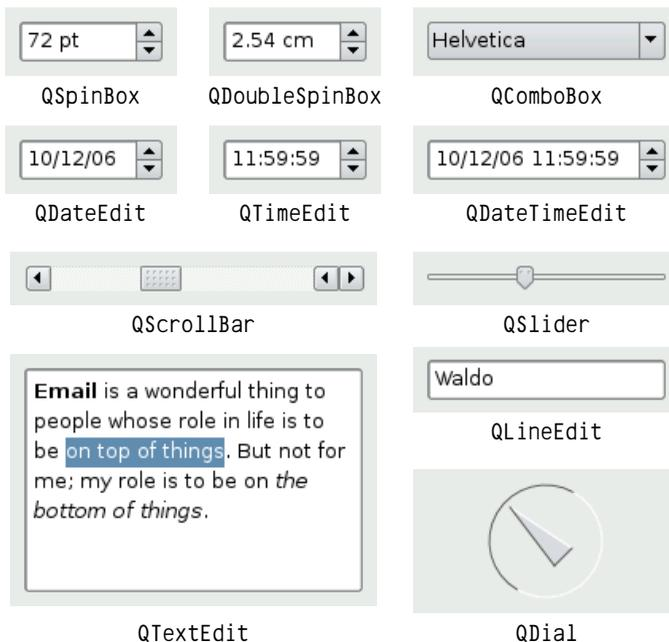
**Figure 2.21.** Qt's input widgets
